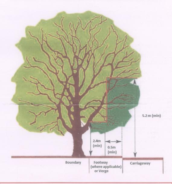
A minimum clearance height of 5.2 metres (17 feet) is required above the carriageway; this height must be continued 0.5 metres (1.6 feet) past the edge of the carriageway.
